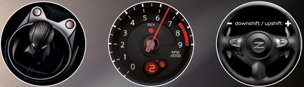
A world's first. Included on the Sport models, SynchroRev Match technology – the first in any production car – monitors the 6-speed manual's clutch pedal, shift lever, and vehicle speed. As you shift to a lower gear, the system will "blip" the throttle to the ideal engine rpm for a supremely smooth downshift as you let out the clutch. The system also works when upshifting to give you a smooth flow of power when accelerating.
